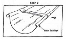
Two 1/8 pilot holes are provided - screw or rivet may be attached through the gutter back from either side. It is not necessary that the holes be aligned. It is important that the fastener is secured through the hanger and gutter back.
