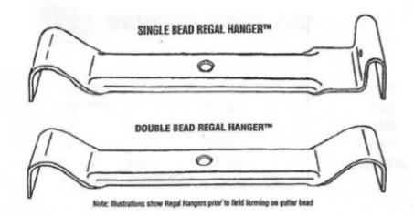
The Regal Hanger will replace the Imperial Style Hanger with a more positive fastening option on the Single and Double Bead Style Gutters. It is available in Mill Finished Aluminum, Galvanized Steel, Copper in 5", 6", 7" and 8". The Regal Hanger Includes an Adjustable Roof Rod and Upper/Lower Hex Nuts.
